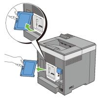
4 Remove the wireless adapter from the printer by releasing the adapter's hook while pushing the wireless adapter towards the front of the printer.
